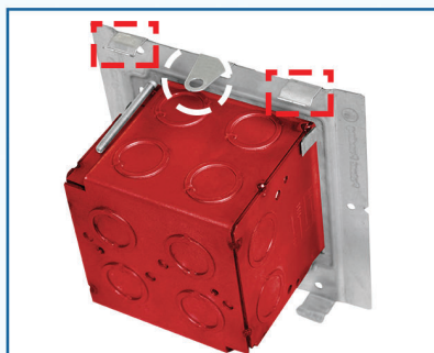
ADAPTER TO BRACKET LOCK Fold tabs to secure adapter on SSB Brackets
