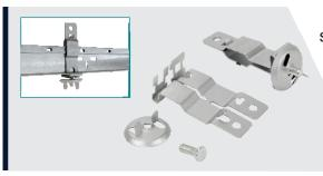
Independent Acoustical Support Clips provide a means to support lighting fixtures from common 15/16" T-grid ceiling channel. ISC requires no tools to install and can support fixtures 65 lbs. or under. Each ISC kit includes a break apart T-grid perimeter clip which cinches both sides of the channel and includes pre-punched holes for branch line restraints. Also includes 5/8" long screw and washer-wingnut.
