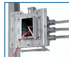
Shown installed to UMA-LVBS* attached direct-to-stud, used as a home run box (* Permits use of 4" rings with 5" box)
