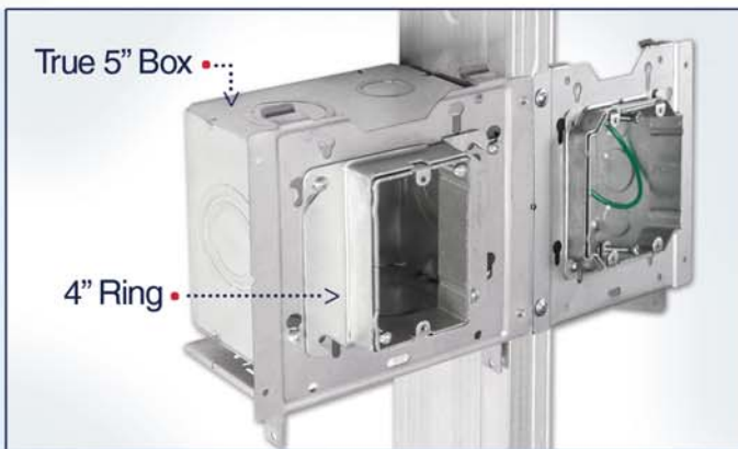
Universal Mounting Adapter w/ Back Support (UMA-LVBS) mounts 4", 4-11/16" and 5" Sq. Boxes direct-to-stud, or snaps onto the SSB-T5 for between stud installations.
