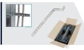
Cable Supports with Locking Tabs make it easy to install and secure NM, AC, or MC-type cables to stud frames. CS-CJ6 reliably supports up to 6 runs of NM cables; or up to 4 runs of MC/AC cables. CS-CJ6 features flared edges for wire protection, locating ribs to keep cables separate, and collapsible locking tabs to secure cables. Helps comply with NEC 300.30(b). Neat, efficient packaging ensures individual pieces can be taken out of the box quickly, without linking together.
