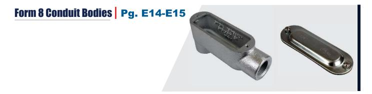
Form 8 Gray Iron Conduit Bodies feature longer bodies and larger wire-pull openings than Form 7 Bodies of the same trade size. This greater size accommodates heavier, larger gauge conductors. Form 8 Conduit Bodies also feature a flat-back design and tapered conduit hubs. Stamped Steel and Gray Iron Covers with integral gaskets are sold separate, and include stainless steel screws.
