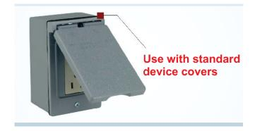
PUT KNOCKOUTS WHERE YOU NEED THEM Field Modifiable Weatherproof Boxes allow installers to drill a KO along the edge of the box by simply using a circle drill. Embossed guidelines assist with positioning. Boxes can be used with existing device covers making them a must-have on every Service Truck!
