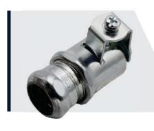
Tubular Steel Double-Bite Compression Combo Couplings also feature a saddle-type clamp, offering all the same advantages of its set screw counterpart above. However, this model features a compression nut in place of a set-screw so there is no risk of seizing screws, dropped screws, or bent EMT raceway. Zincplated steel design offers a higher tensile strength than common zinc die cast combo fittings. For dry locations only.
