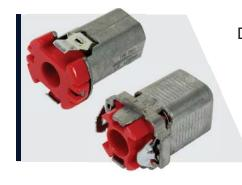
Double-Snap Connectors work to make terminating AC/MC cables to steel boxes and enclosures easy and tool-free. Available for both new and old-work installations, each connector can be assembled to the cable or box without tools, resulting in a much faster installation. Both fittings are also easily removable and re-usable.
