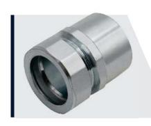
Steel Rigid to EMT Compression Combo Couplings improve upon more common set-screw type combination fittings. One end of the coupling is threaded for 1/2" thru 1" Rigid/IMC conduit; the other end is un-threaded for 1/2" thru 1" EMT. Unlike set-screw fittings, the SREC Series greatly reduces the risk of seizing screws, or the accidental bending of EMT due to over-torque. Compression type fittings are also wet location or concrete rated.
