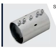
Steel EMT slip couplings with set-screw type connections are commonly used to join two EMT conduits together. The unique center screw design allows for a seamless fit, eliminating the need for flex conduit between the prefab conduit racks. This feature not only saves time during prefabrication in the shop but also increases productivity in the field. Additionally, the steel construction provides mechanical protection and a secure connection between the conduits.
