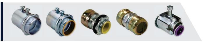
Steel Fittings offer a higher tensile strength and higher yield strength than Zinc Die-Cast Fittings. Machined from a solid bar of stock steel, Steel Fittings are coated with zinc plating for corrosion protection. Steel Fittings are suitable for dry and/or wet locations, and are considered to be "specification grade" fittings.
