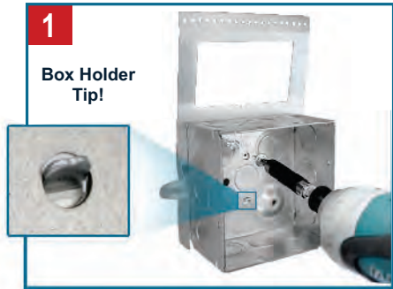
Attach to a 4" or 4-11/16" box with a single wafer head screw, forming a versatile box assembly
